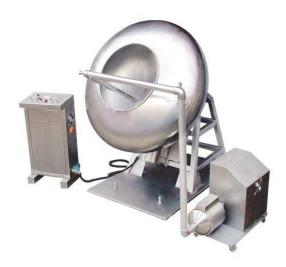
Coating Machine is available with 12", 24", 30", 36", 42", 48", 60" or 72", size SS Pan. Coating Machine is totally enclosed with MS Cladding with standard Gear Box, Motor, Hot Air Blowing arrangement. Machine is designed with MS fabricated structure and all arrangement – except electric control, air filter and SS Pan are inside the enclosure, which makes simple cleanable outside covering. Machine is mounted on dynamounts which avoids foundation.
